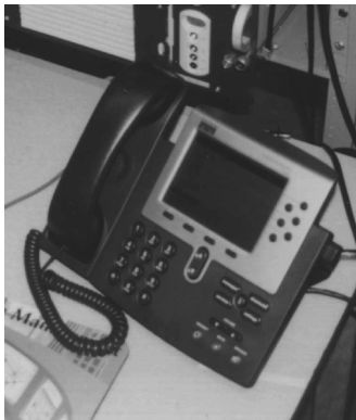
Voice over Internet Protocol (VoIP) test phone. Each phone has a unique Internet address.
